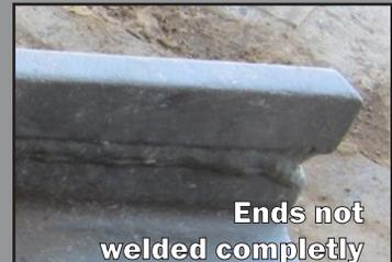
6. It is important to make sure that the ends of the grouser bar are completely welded to the shoe. Don't leave cavities where the weld was started as this will allow the end of the grouser bar to break off. The pictures to the right show examples of poorly welded grouser bar.
