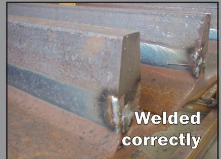
9. It is recommended that amperes and wire feed be set as high as the operator can easily handle. The purpose of this is to achieve a fast low penetration weld procedure helping to prevent Carbon from the grouser bar building up in the weld puddle and making it crack sensitive.
