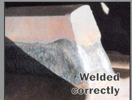
10. Avoid quenching or rapid cooling of welds. Do not let the welds come in contact with water, mud, snow etc.
