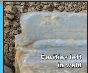
7. Control the bead shape or size of the deposited weld. As the hot
